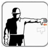
LOWER BOOM HOLD (RAISE LOAD)
