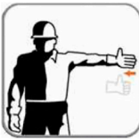
RAISE BOOM HOLD (LOWER LOAD)
