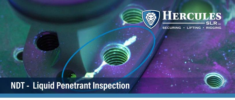
Dye Penetrant Inspection (DPI), also called Liquid Penetrant Inspection (LPI) or Penetrant Testing (PT), is one of the oldest and simplists NDT methods where its earliest versions (using kerosene and oil mixture) dates back to the 19th century. Liquid penetrant inspection is used to detect any surface-connected discontinuities such as cracks from fatigue, quenching, and grinding, as well as fractures, porosity, incomplete fusion, and flaws in joints.
